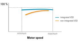
• Special attention is given to the electric motor, which is specifically designed for VSD operation (inverter duty motor). Bearings are protected against induced bearing currents and both motor and converter are perfectly tuned to obtain the highest possible efficiency over the entire speed range.
