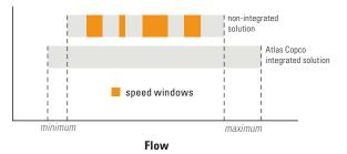
The machine is tested for the complete speed range to eliminate any 'speed windows' that could jeopardize the energy savings and the stable net pressure. (Turndown capability of the compressor is maximized to 80-85%.)
